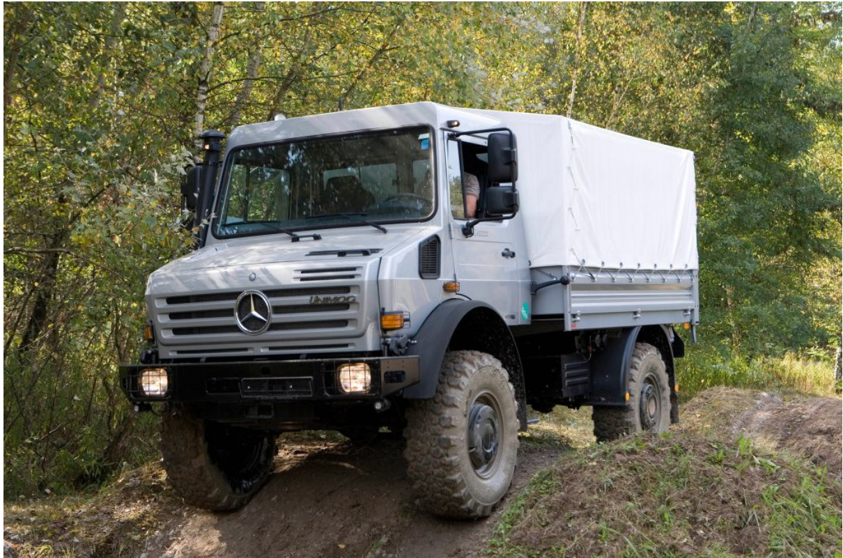
Figure 11: The Unimog is being investigated as a possible tool carrier to mount the twin chop forage harvester or a flail plus vacuum lift such as in figure 9.
