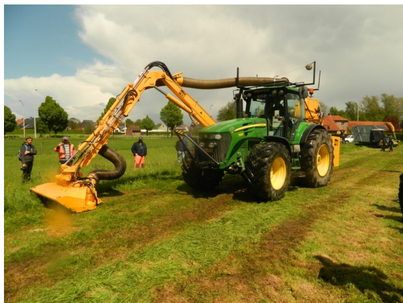
Figure 10a: Herder 'Eco' Rotary Mower with vacuum pick up – a flail mower version is in common use across parts of France, Holland and Belgium. The unit can have a collection trailer attached.
